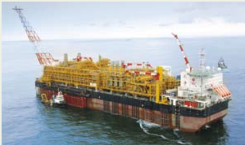
The Dalia FPSO vessel is 300 meters long and 60 meters wide, with accommodations for up to 190 people.
